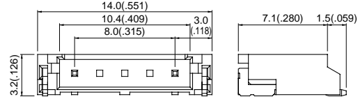
(2 circuits 8.0mm(.315")pitch plugged up)
