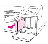
5. Remove the ink cartridge from the bag. Shake the ink cartridge for approximately five seconds, and 15 times, horizontally.
