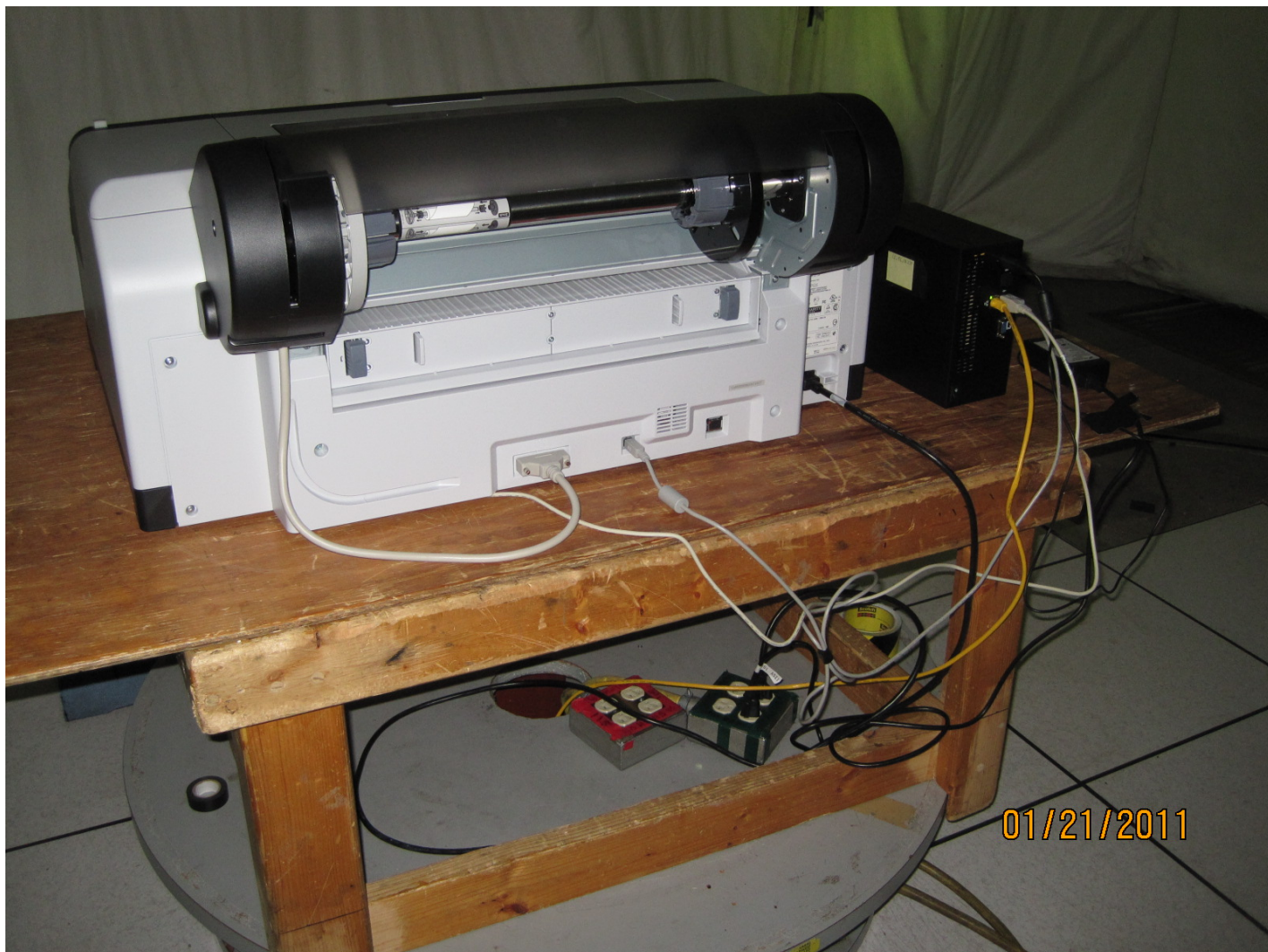
Test-setup photo(s): Radiated Emissions 30 - 8000 MHz
