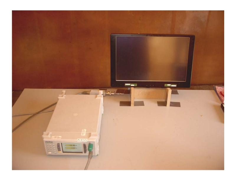
Maximum Peak Output Power Measurement Setup
