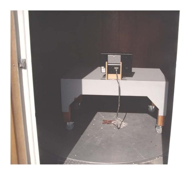
Radiated Emissions Measurement (Rear View) Setup
