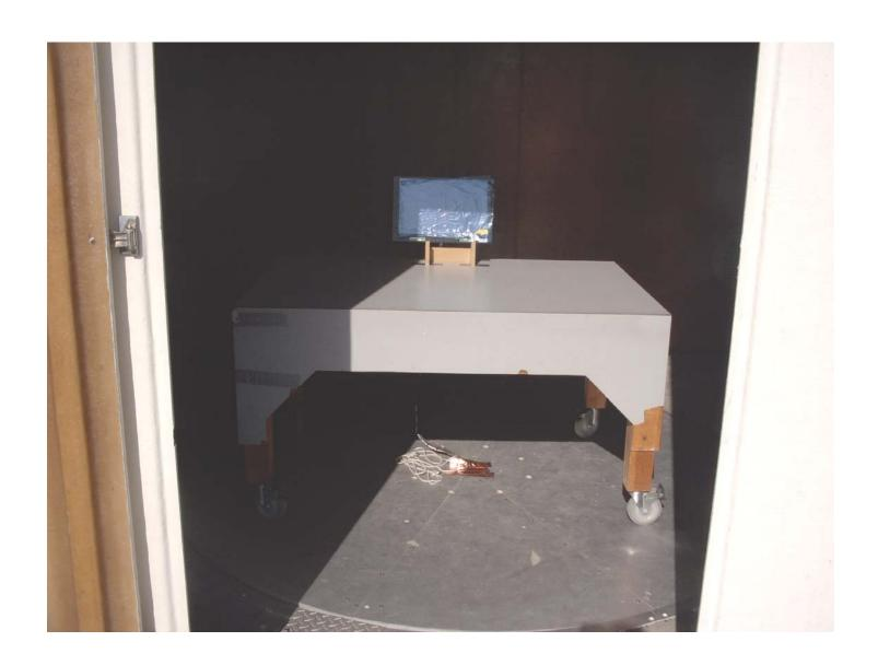
Radiated Emissions Measurement (Front View) Setup
