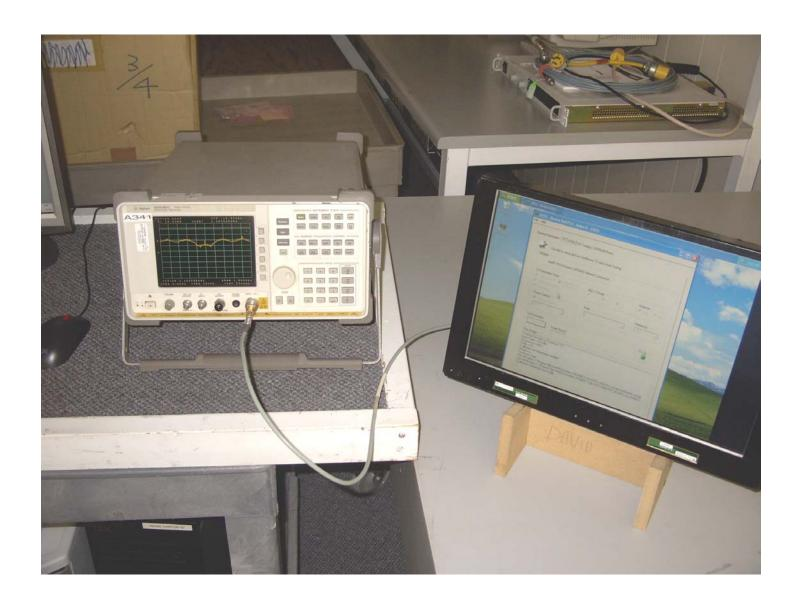
Conducted Emissions at Antenna Terminal Setup
