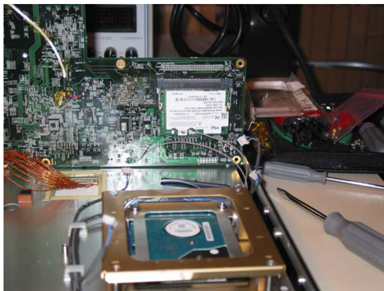
RF Module Installed in Unit
