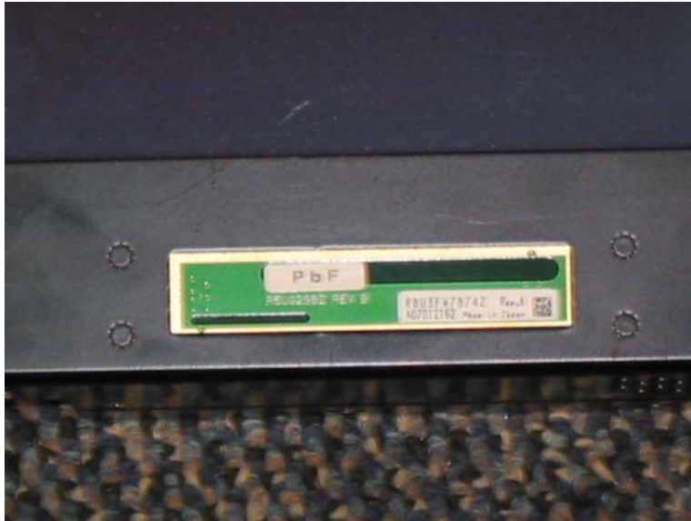
Close Up of Antenna
