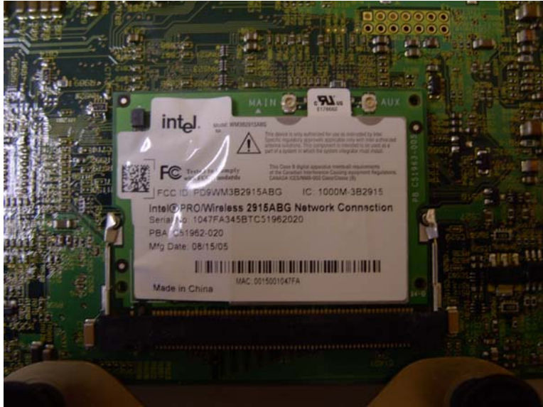
Module Installed in PSEB
