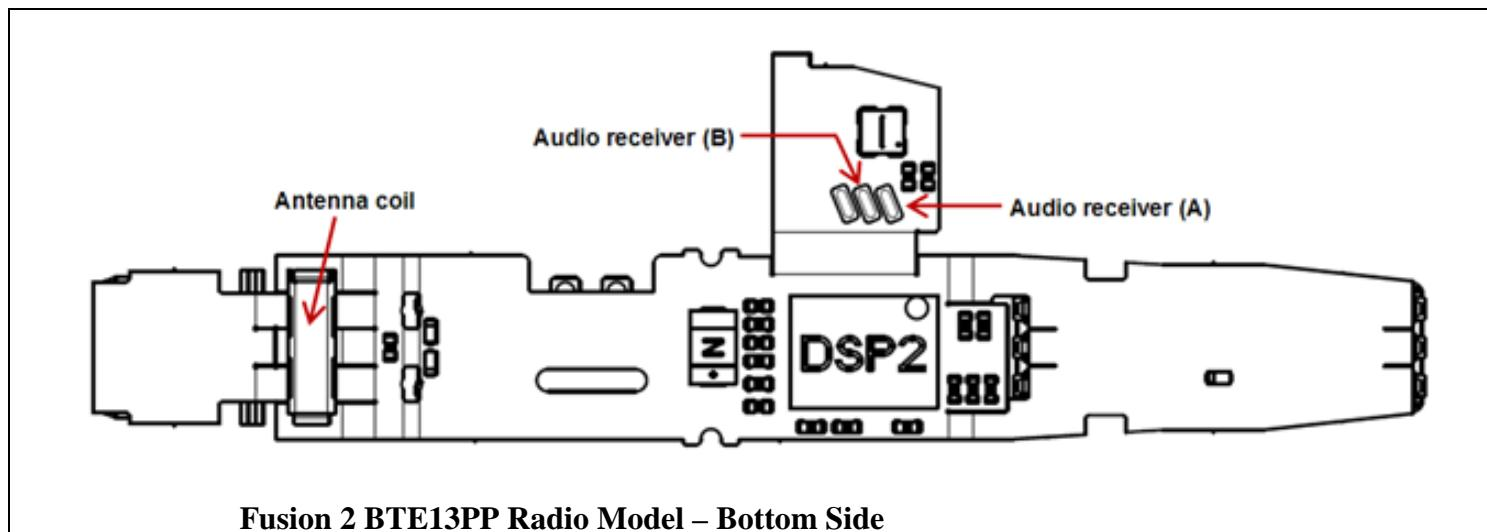
On the bottom side of the radio model the DSP, the antenna coil and pads for connecting the audio receiver can be seen.
