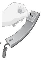
Not all telephones can activate the Auto Telephone. The telephone receiver may need to have a special magnet fitted. Please follow the separate instructions for mounting the magnet, which are available from your hearing care professional.
