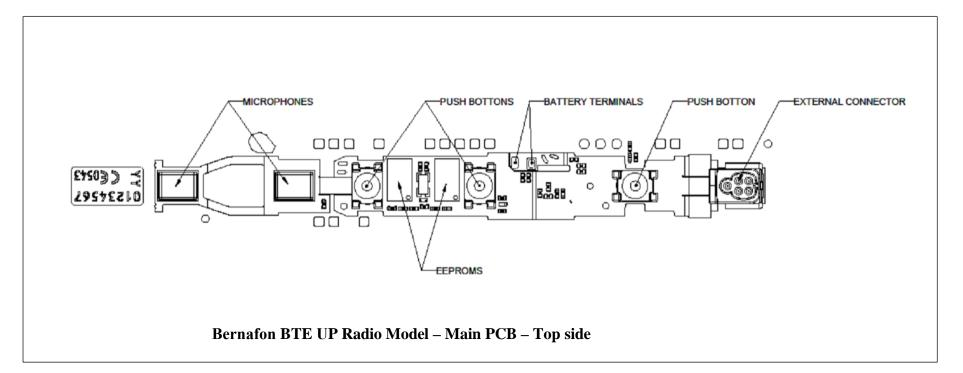
The most important part of the radio model is the Engine Module mounted on the main flex PCB, which connects it to both the EEPROM memory and all external connections: On the top side these are the microphones, the battery terminals and the push button. The telecoil is also used for wireless battery charging.
