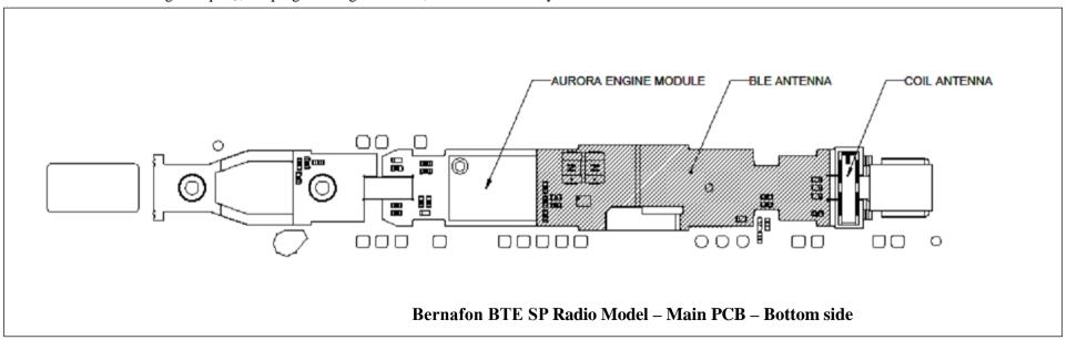
The most important parts inside the Engine module are a Digital-Signal-Processor (DSP), a radio Front-End (FE) chip for the 3.84 MHz radio part and an RF chip for the Bluetooth radio part – all mounted on a small rigid PCB again mounted on the main flex PCB. The Bernafon BTE SP radio model also includes all voltage regulators and buffered data programming inputs on board. The DSP is the main processor controlling the functionality of both radios in the Bernafon BTE SP radio model.
