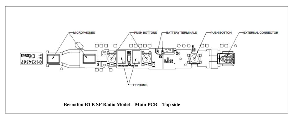
The most important part of the radio model is the Engine Module mounted on the main flex PCB, which connects it to both the EEPROM memory and all external connections: On the top side these are the microphones, the battery terminals and the push button. The telecoil is also used for wireless battery charging.
