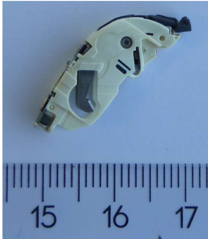
Right side with battery interface clip
