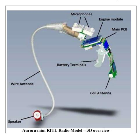
The radio model is implemented in an engine module mounted on the main PCB with connections to the antennas, the microphones, the speaker and the battery terminals. The radio model can be seen in 3D overview to the left:
