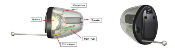
The Aurora CIC radio model is intended to be installed in Bernafon wireless CIC hearing aid devices (Completely-In-the-Canal) styles.
