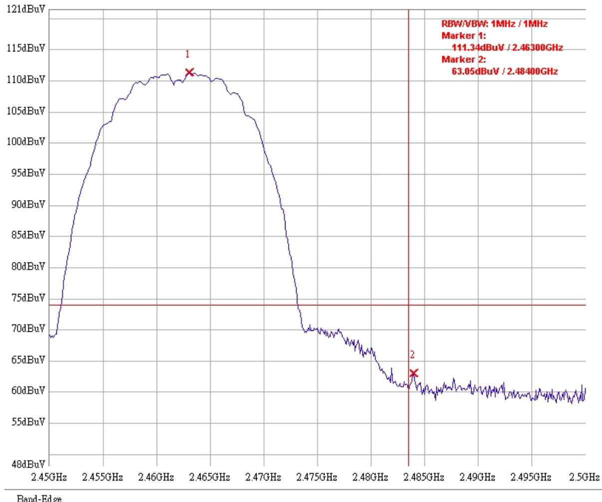
**Test Mode: 802.11b mode (CH 11 AV)**
