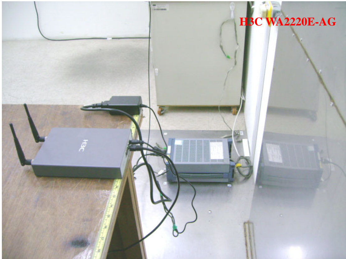
Photo 2: Conducted Emission Test Set-up photo
