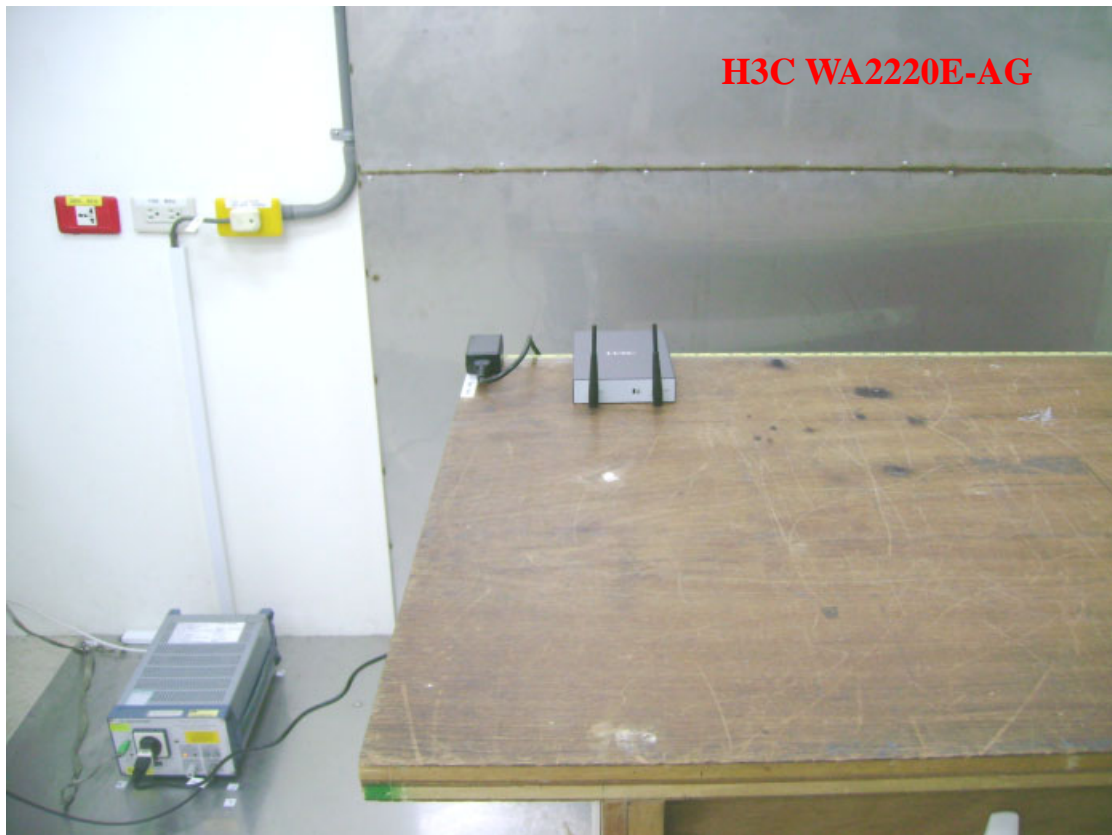
Photo 1: Conducted Emission Test Set-up photo
