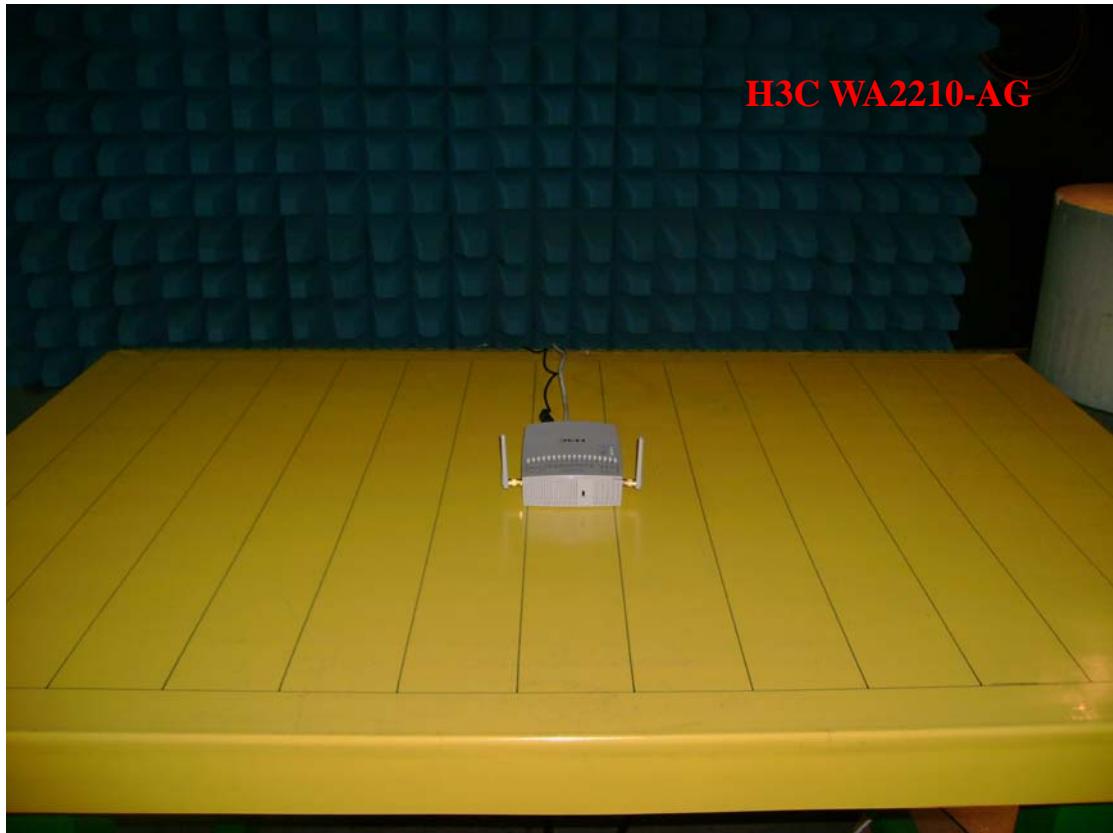
Photo 2: Radiated Emission Test set-up photo
