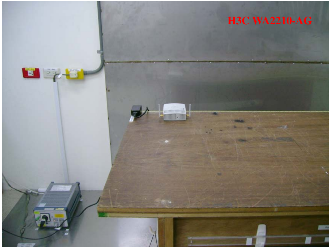
Photo 1: Conducted Emission Test Set-up photo
