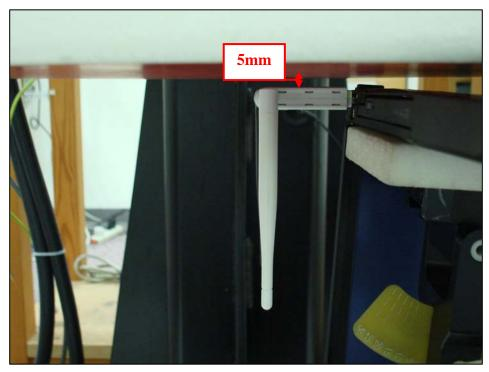
(1-2) Horizontal Down Up90(10 mm separation from the flat phantom for the end of the dongle (opposite from the USB connector))
