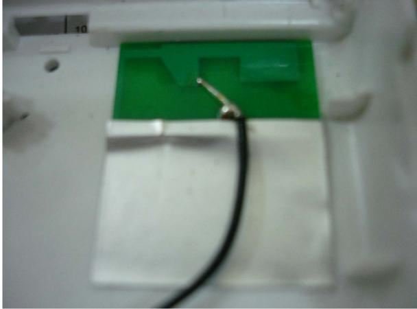
Antenna Gain: 2dBi (Manufacture: BRITO TECHNOLOGY)
