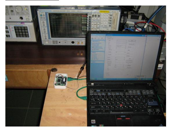
POWERLINE CONDUCTED EMISSIONS MEASUREMENT SETUP
