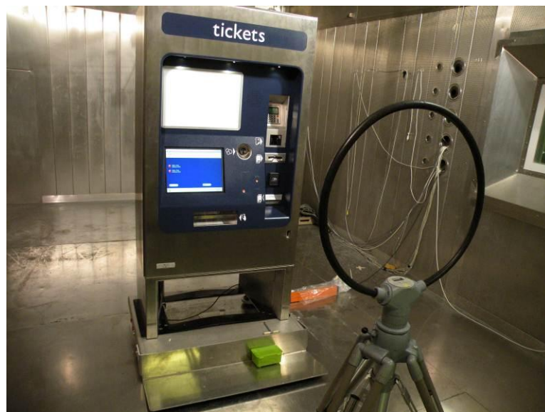
Photo 4: H-Field Measurement in the climatic chamber
