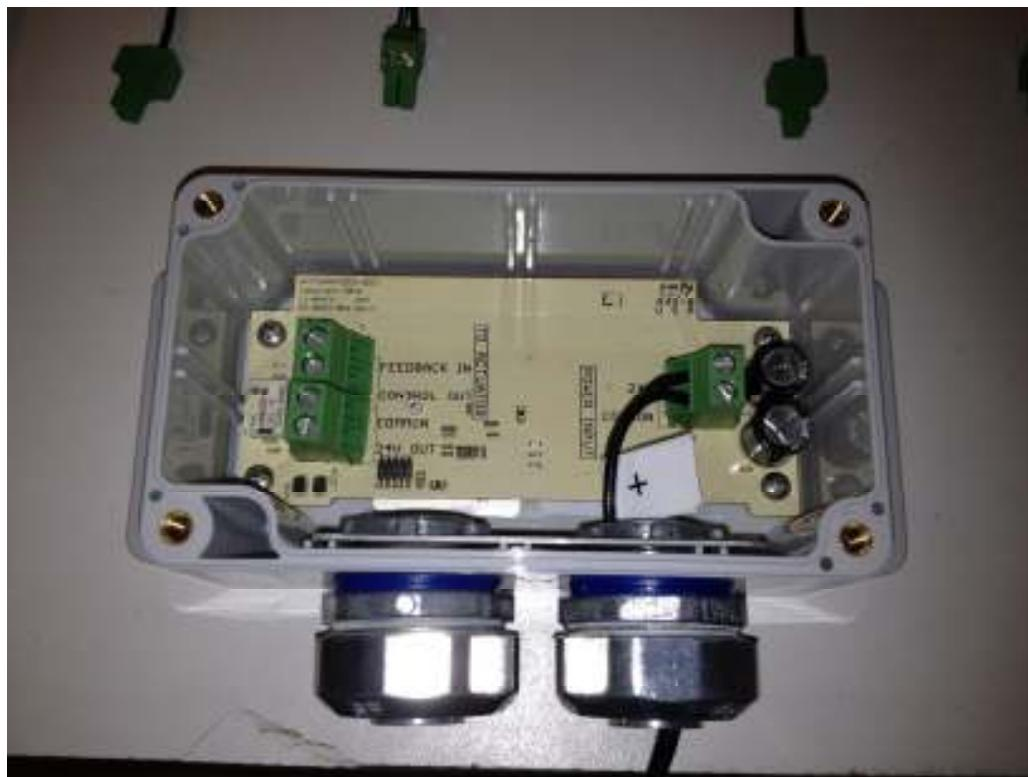
Once all connections are complete, the clear top lid should be replaced and screwed in tightly. When using the provided watertight conduit connectors, the enclosure supports NEMA4X certifications if properly tightened using the specified torque rating of 8 in-lbs.
