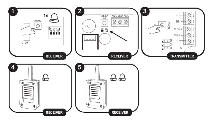
If 10 seconds pass without programming a transmitter, the receiver will exit the programming mode.
