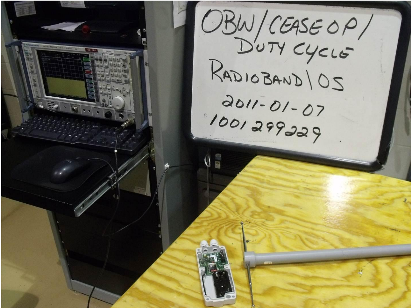
Figure 1 Test Setup for Occupied Bandwidth
