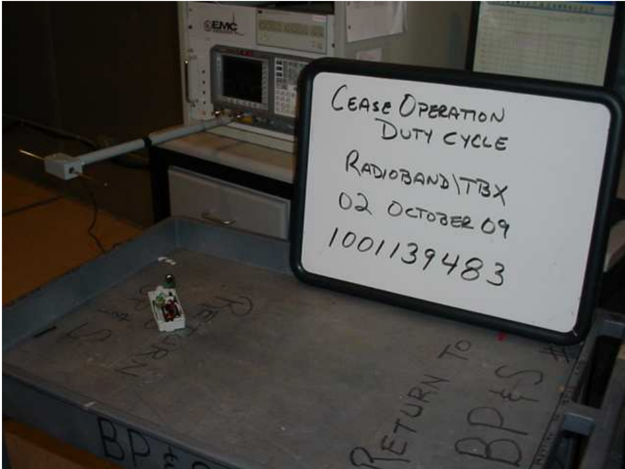
Figure 6 Test Setup for Pulse Train
