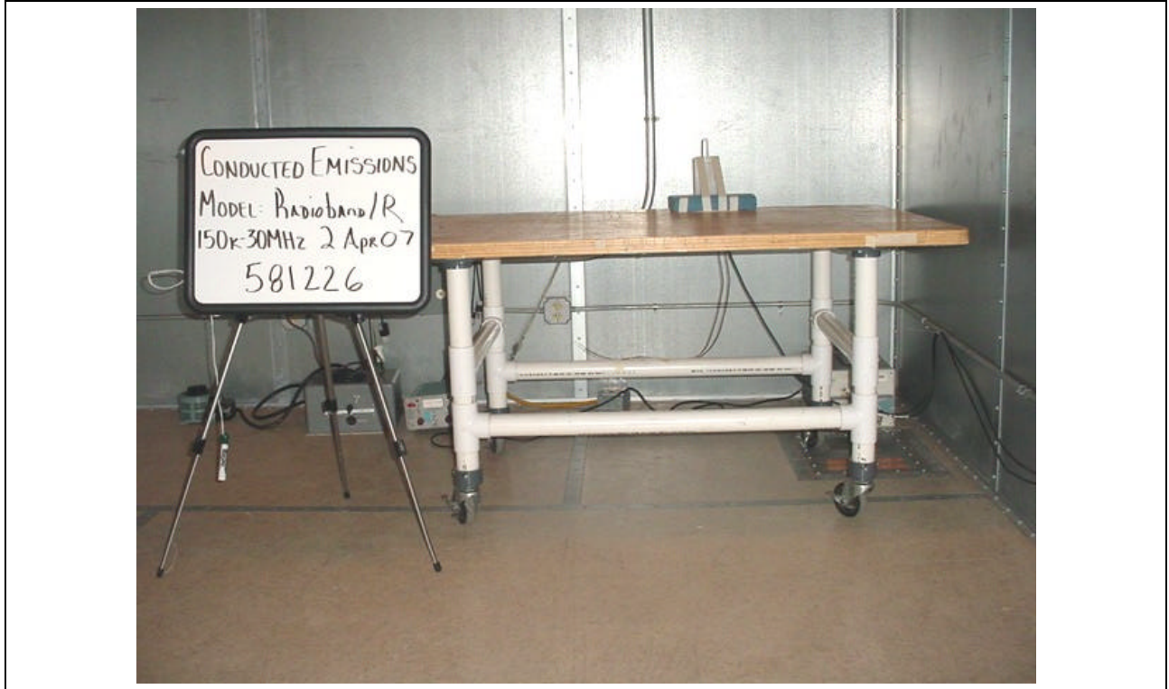
Figure 8 Test Setup for Conducted Emissions
