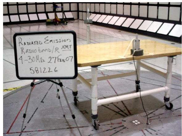
Radiated Emissions Setup 4-30MHz XMT Mode
