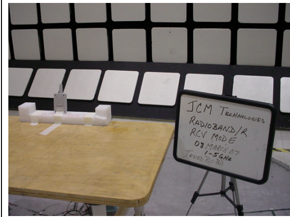
Radiated Emissions Setup 1-5GHz RCV MODE
