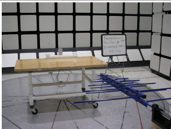
Radiated Emissions Setup 30-1000MHz XMT MODE
