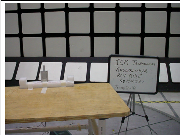
Radiated Emissions Setup 30-1000MHz RCV Mode
