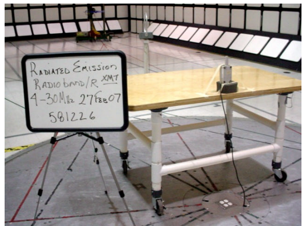
Radiated Emissions Setup 4-30MHz XMT Mode
