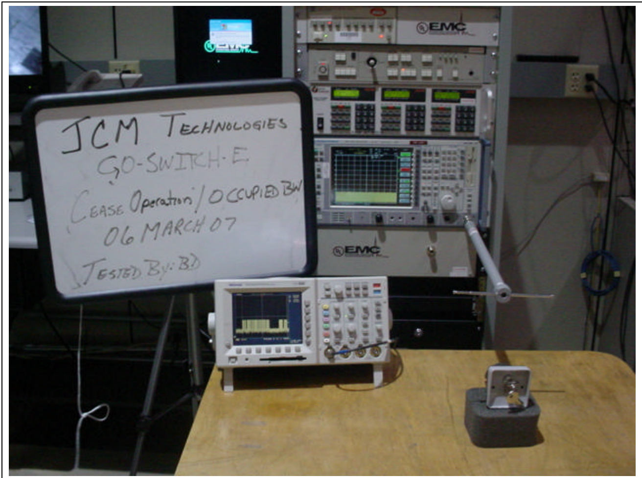
Figure 12 Test Setup for Occupied Bandwidth
