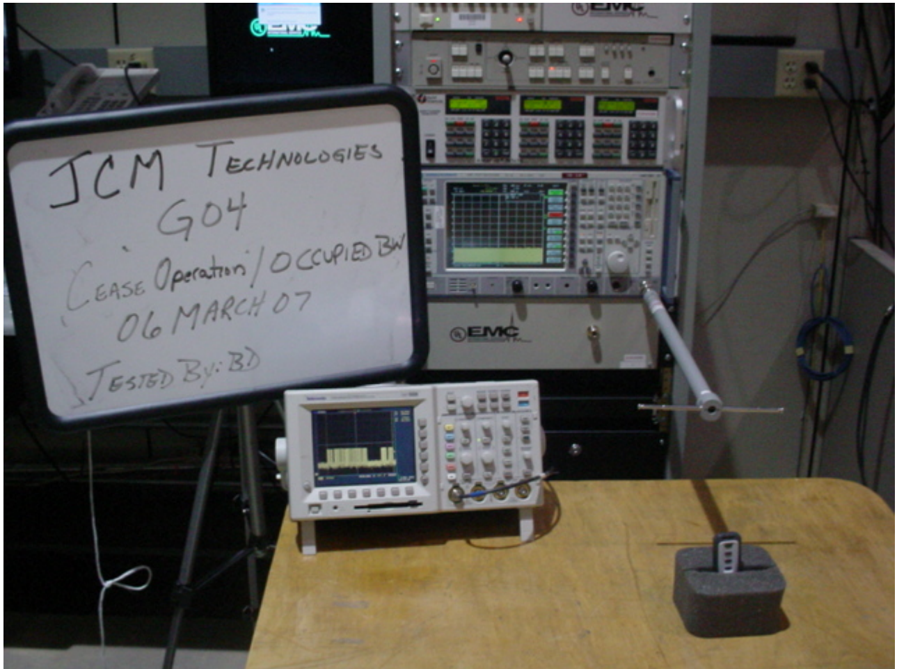
Figure 8 Test Setup for Cease Operation
