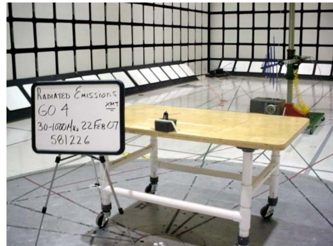
Figure 13 Test setup for Radiated Emissions – 30-100MHz – Front and Rear Views
