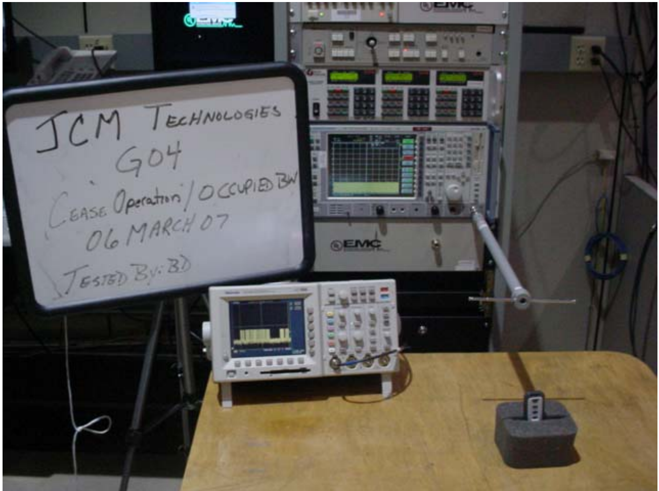
Figure 10 Test Setup for Occupied Bandwidth
