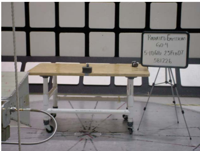
Figure 15 Test setup for Radiated Emissions – 5-10GHz – Front and Rear Views
