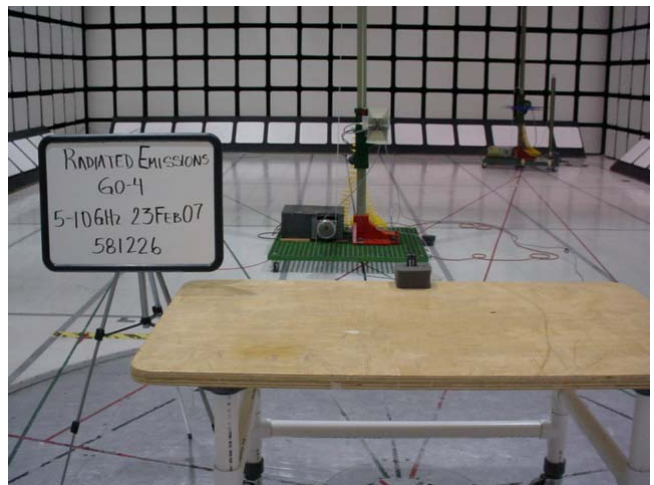
Figure 15 Test setup for Radiated Emissions – 5-10GHz – Front and Rear Views
