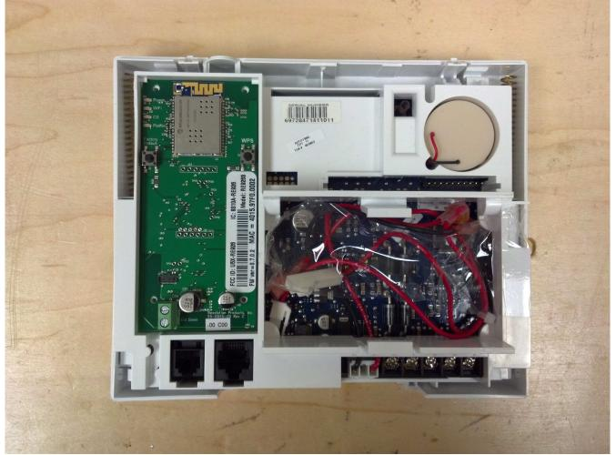
12. The above picture shows the correct installation of the RE926S in the back of the SimonXT.
