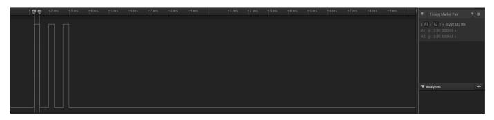
The radio has a capability of transmitting 3 advertisement packets at a minimum interval of 20ms or 1 connection packet every 7.5ms. The worst case being 3 packets in a 20ms window. Converting the timing over a 100ms window shows that the radio is well below the 10ms in a 100ms window for maximum duty cycle correction.
