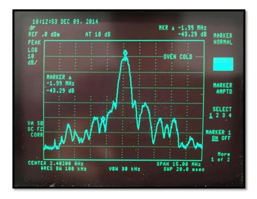
The following plot shows the fundamental and the level at the highest spur beyond the band edge. The level at the highest spur beyond the band edge is 39.99dB down from the fundamental.
