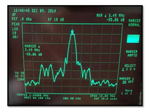
The following plot shows the fundamental and the level at the highest spur beyond the band edge. The level at the highest spur beyond the band edge is 51.26dB down from the fundamental.
