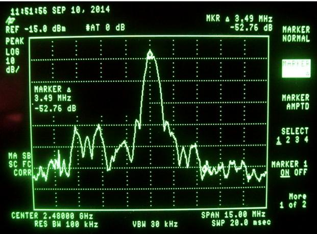
The following plot shows the fundamental and the level at the highest spur beyond the band edge. The level at
