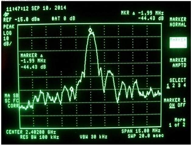
The following plot shows the fundamental and the level at the highest spur beyond the band edge. The level at the highest spur beyond the band edge is 39.71dB down from the fundamental.
