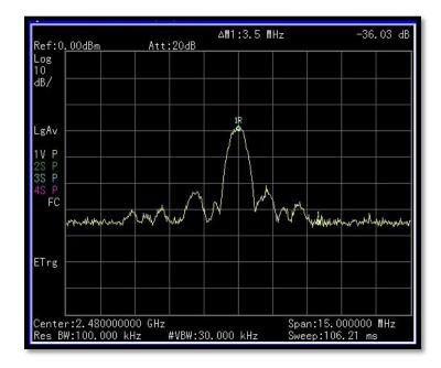
The following plot shows the fundamental and the level at the highest spur beyond the band edge. The level at the highest spur beyond the band edge is 32.73dB down from the fundamental.
