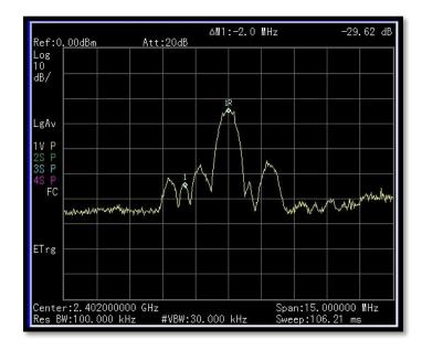
The following plot shows the fundamental and the level at the highest spur beyond the band edge. The level at the highest spur beyond the band edge is 26.69dB down from the fundamental.
