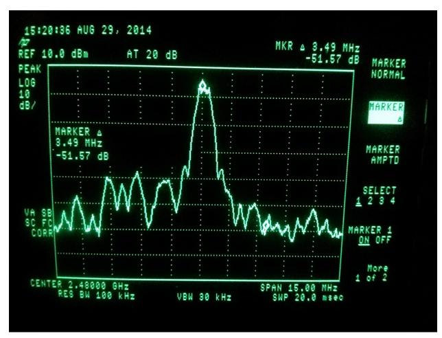
The following plot shows the fundamental and the level at the highest spur beyond the band edge. The level at the highest spur beyond the band edge is 43.34dB down from the fundamental.
