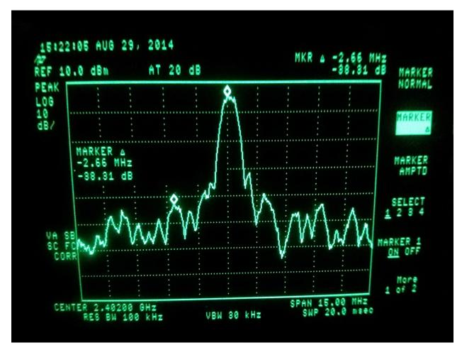
The following plot shows the fundamental and the level at the highest spur beyond the band edge. The level at the highest spur beyond the band edge is 38.31dB down from the fundamental.
