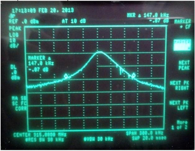
Resolution Bandwidth: 30kHz Video Bandwidth: 30kHz
