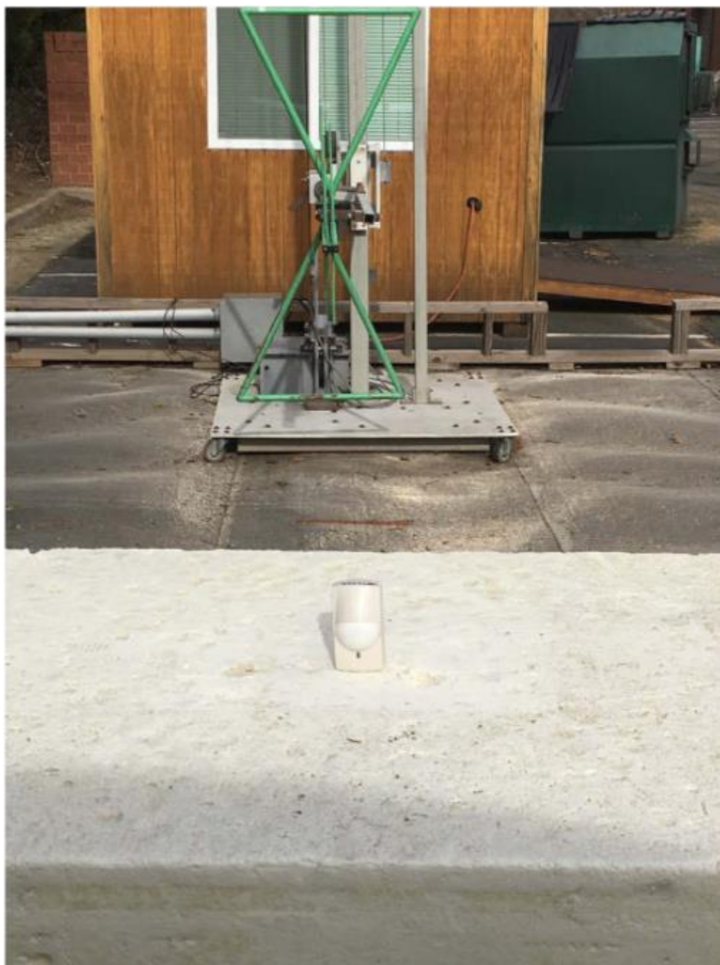
Radiated Emissions (Less Than 1 GHz)
