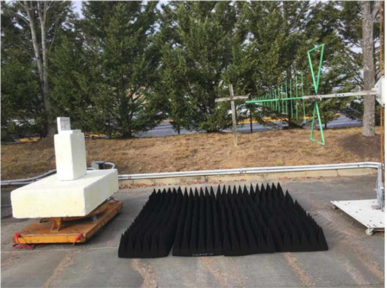
Radiated Emissions (Greater Than 1 GHz)
