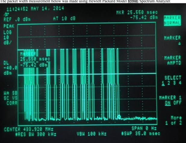
The packet width measurement below was made using Hewlett Packard Model 8594E Spectrum Analyzer.
