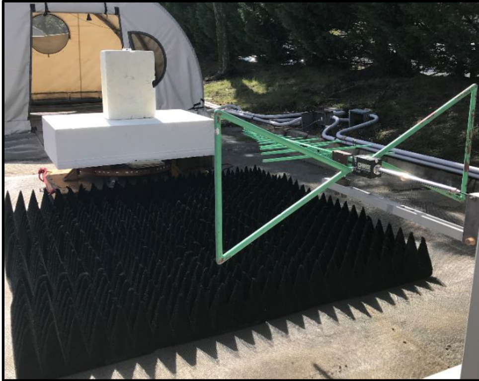
Photograph: Radiated Emission, Above 1 GHz, Front
