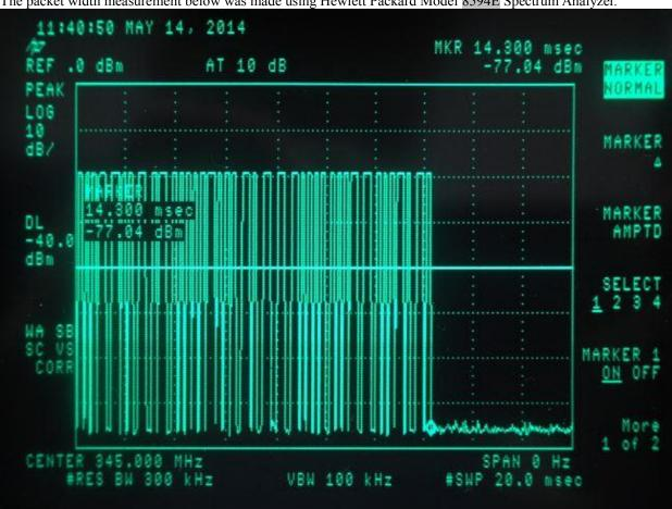
The packet width measurement below was made using Hewlett Packard Model 8594E Spectrum Analyzer.
