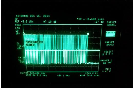
Calculating the allowed duty cycle correction factor as given in §15.35(c):
