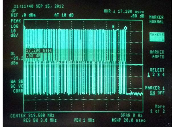
The packet width measurement below was made using Hewlett Packard Model 8591E Spectrum Analyzer.
