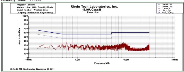
Client: Resolution Engineering Model: 56-0042-01 WIRELESS SIREN 433.9 MHz FCC ID: N/A Standards: FCC Part 2, 15
