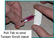
3. The tamper enrollment signal can be re-sent by touching a magnet to the sensor 5 times within 5 seconds.
