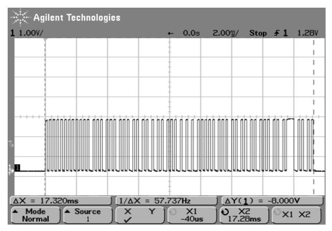
Calculating the allowed duty cycle correction factor as given in §15.35(c):
