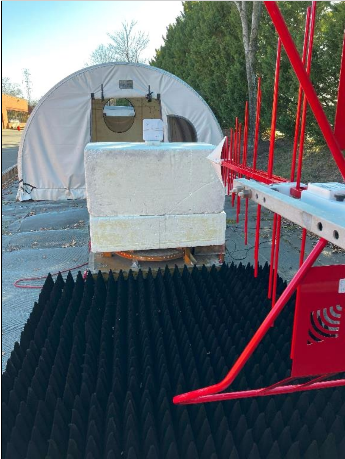
Photograph 3: Radiated Emissions, Above 1 GHz, Front
