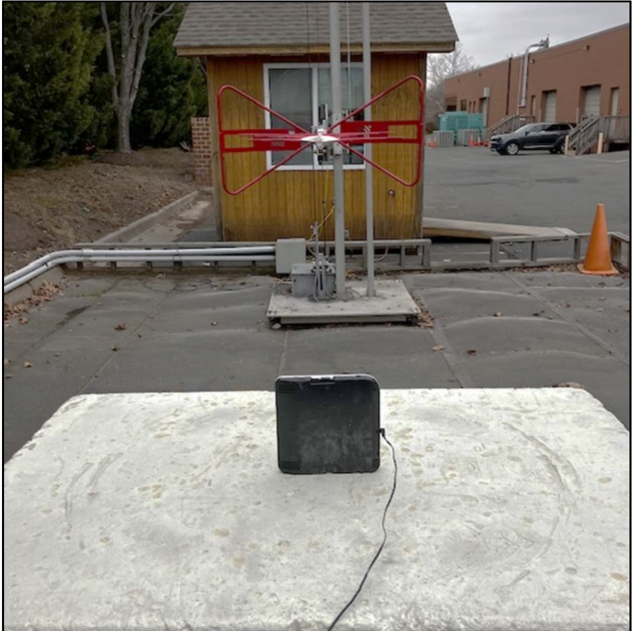
Photograph 2: Radiated Emissions, 30 MHz – 1 GHz, Rear
