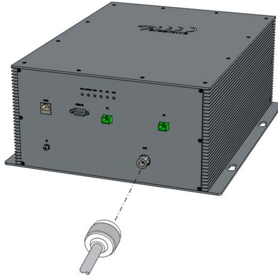
Figure 3-4 RAM2241 RU power supply connection
