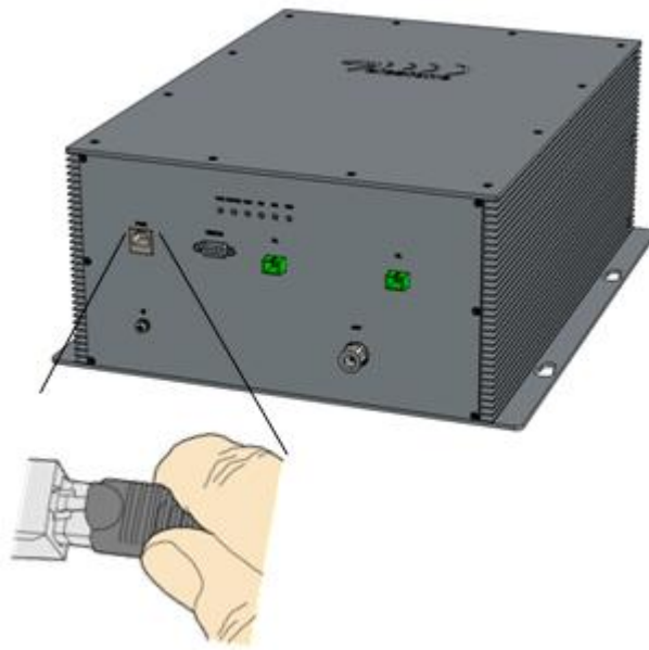
Figure 3-6 RU power line cable connection
