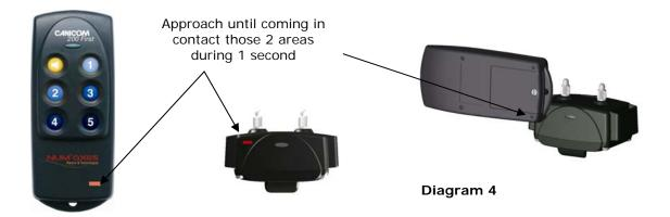
To increase the battery life of the remote control and receiver collar, you should deactivate the units if you are not using them for a long period.
