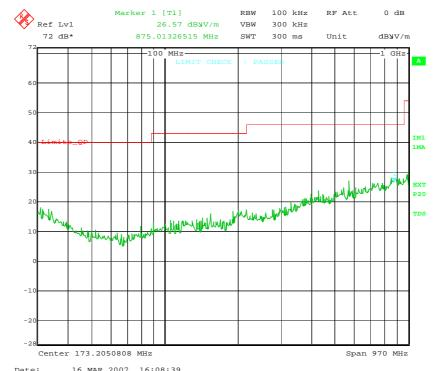
For noise floor plot, video averaging is done with a  $1kHz\ VBW$  which is sufficient to show a noise floor more than 6dB below the limit.
